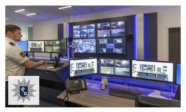
The newly created workstations in the <u>Bremen Police Department's video control center</u> were installed according to the latest ergonomic principles. This includes, for example, an electromotive height adjustment of the control room consoles, which allows different users on 24/7 shift duty to adjust the Stratos desk to individual needs.
