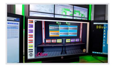
JST MultiConsoling®: The monitor displays the myGUI user interface for the MultiConsoling®. Good to recognize: Whereas previously only one console was used per workstation, thanks to the positive experience with the innovative JST technology, this has now been increased to a total of three consoles per workstation, i.e. each screen in the s.Oliver control center now runs via MulitConsoling®.
